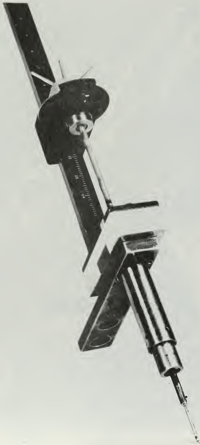
FIGURE 16 THREE-HOLE PROBE DETAIL
